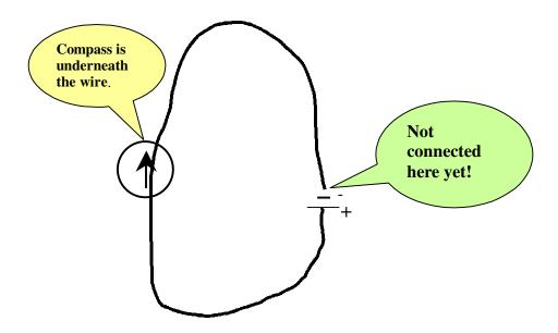
5. Briefly connect the wire to the negative end of the battery and watch what happens to the needle on the compass. Draw the needle in the next diagram exactly how it appears when the circuit is closed. (Wire is connected).
