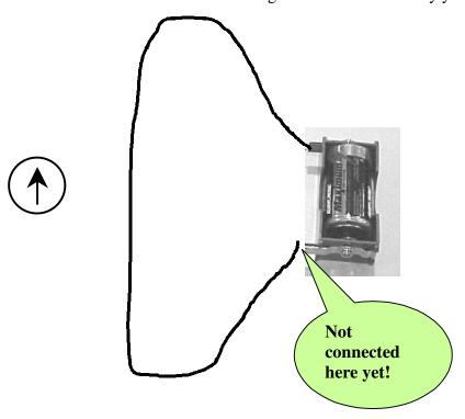
2. Move the compass in such a way that it is underneath the wire and the needle is pointing parallel to the direction of the wire. Since compasses point North, you may have to rearrange the battery and the wire in order to do this. Don't connect the wire to the negative end of the battery yet.
