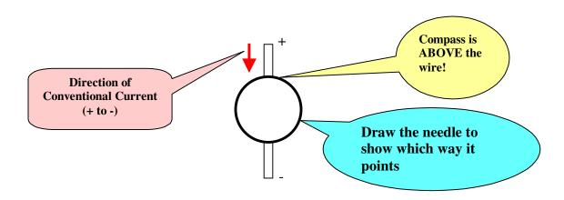
8. **Flip the battery** so that the positive and negative ends are switched. Move the compass in such a way that it is **above** the wire and the needle if pointing parallel to the direction of the wire. Don't connect the wire to the negative end of the battery yet.
