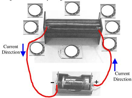
When the <u>current</u> through a coil is reversed, the direction of the magnetic lines of force
