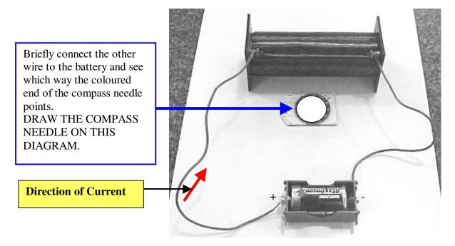
As soon as you see which way the needle points, disconnect the wire from the battery.
