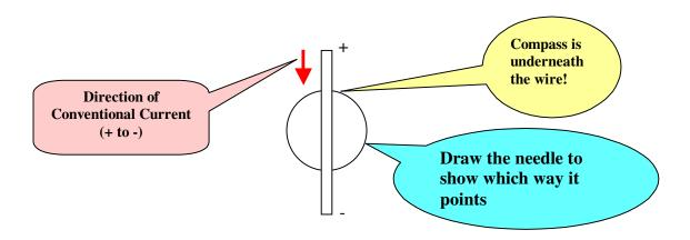
4. **Flip the battery** so that the positive and negative ends are switched. Move the compass in such a way that it is underneath the wire and the needle if pointing parallel to the direction of the wire. Don't connect the wire to the negative end of the battery yet.
