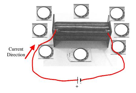
18. Now disconnect the battery and <u>reverse it</u> so that the + is on the right side and move the compass to the positions shown in the following diagram.
