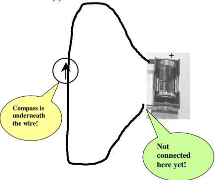
3. Briefly connect the wire to the negative end of the battery and watch what happens to the needle on the compass. Draw the needle in the next diagram exactly how it appears when the circuit is closed. (Wire is connected).
