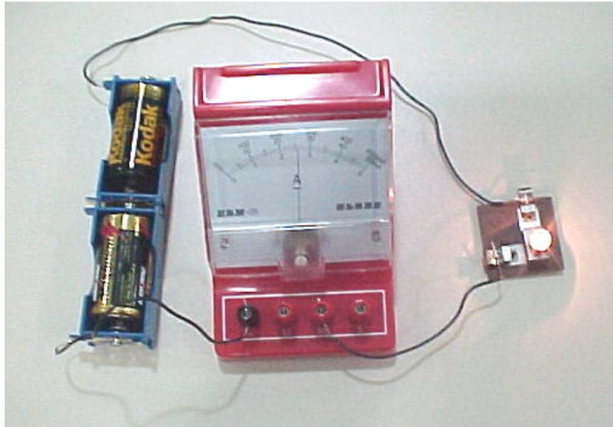
Make sure the **negative** end of the batteries is connected to the **black** terminal on the ammeter. The wire from the **positive** end **MUST** be connected to the **lamp**. The wire from the other terminal on the lamp should be connected to the middle red terminal (eg. the 500 mA range). **Read** the current (I) on the meter in milliamperes (mA) and record it on the schematic diagram on the next page.
