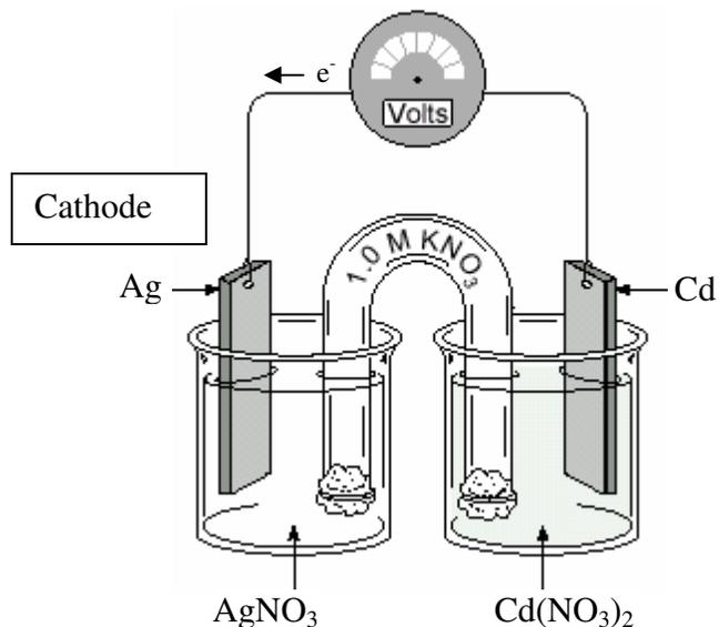
The initial cell voltage is 1.20 Volts
