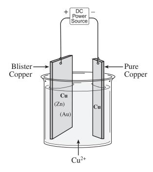
Sufficient voltage is supplied to oxidize copper at the anode.
